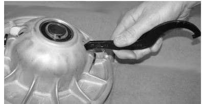
Apply force to opposite end of tool to spread sheaves
