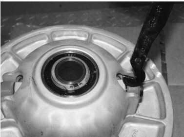
Insert hooked end of tool
