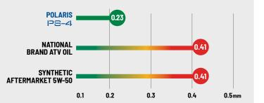
ASTM D4172. In 3rd party testing against 9 competitive products Polaris had 40% or better wear protection compared to all of The tested products. Numbers represent more fiver scarcing measured. Test measures wear protection compared to all of the tested products. Numbers represent more fiver scarcing measured. Test measures wear at contact point, was rear is measured for its length and width (in units of mm). Lower wear numbers mean better wear protection and friction reduction.
