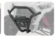
FRONT WINCH BUMPER • Elevated mounting location on bumper for easy access to 4,500 LB Winch • Requires winch (2885127, 2885126), sold separately
