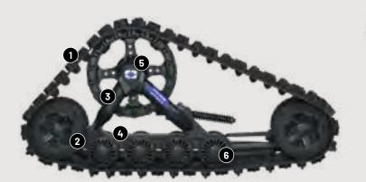
**1** INDUSTRY-FIRST FLEX-TRACK DESIGN Front-mounted tracks with flexible sides and a slight inward curve allow for stable handling, a more comfortable ride and precise steering over long-distances or extended working hours.
